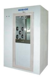
Air shower is a necessary passage for person entering clean room in order to minimize the amount of particulate contaminant, achieve workplace strict clean purification standards. Personnel move through the air shower while particulate contaminants are blew off by the clean high speed air. So the dust can't be brought into clean area.
