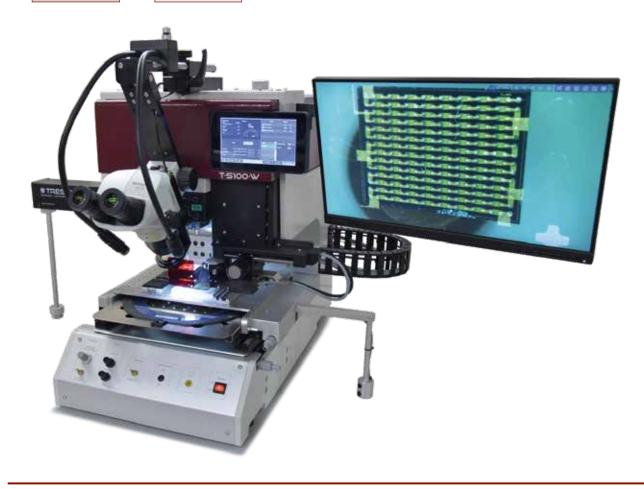
Operating a Tresky die bonder/placer is intuitive. A few minutes' training is sufficient to start working with the machine. The accuracy and repeatability of placing parts is superb thanks to a number of well-thought out features like a true, linear Z-Axis, Force Control, XY Fine Control and high-resolution optics that allow flip-chip placing down to sub-micron accuracy.
