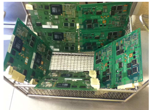
Cleaned PCBAs using DISPER 607
